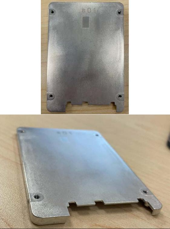
Two photographs of the same metal case after needle barrel polishing. The top image shows the case with a bright, reflective finish and the marking "B 01" at the top. The bottom image shows the case from a different angle, highlighting the smooth, polished surface. |
