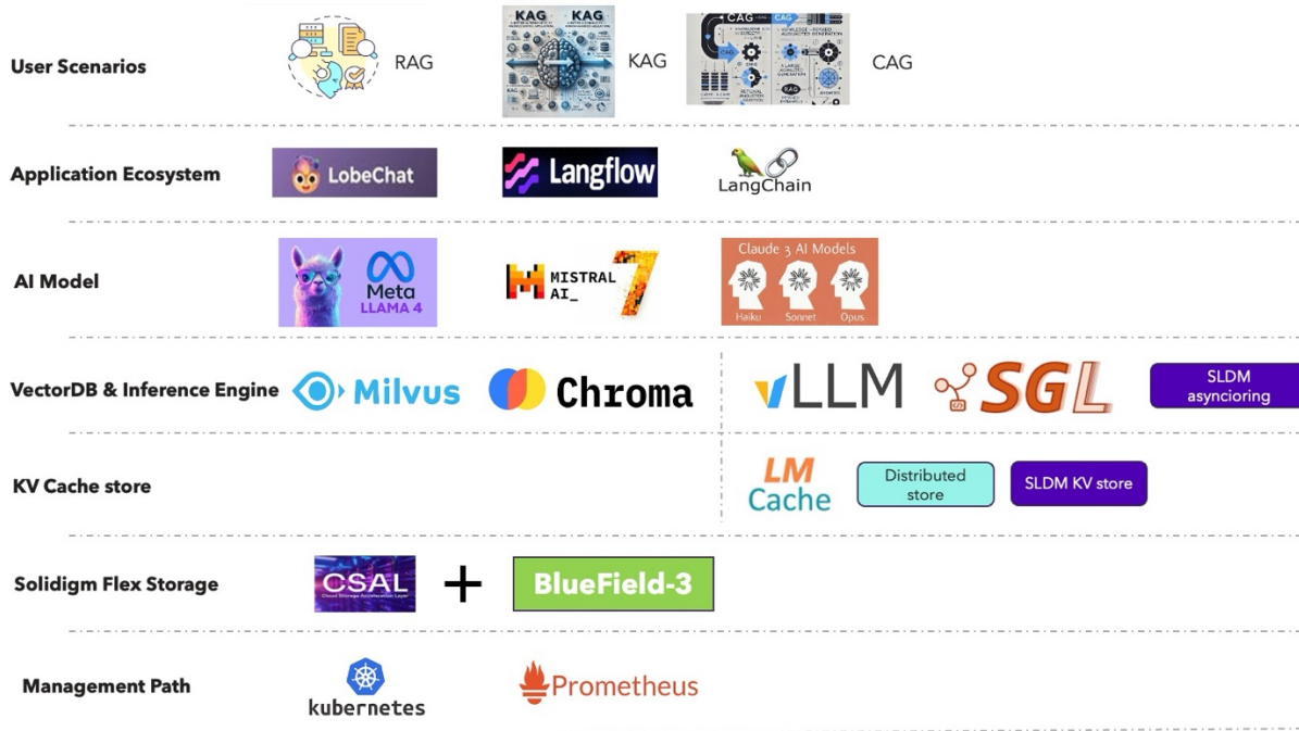
Figure 2-1 An End-to-End View of the LLM Inference Ecosystem with CSAL and Bluefield-3
